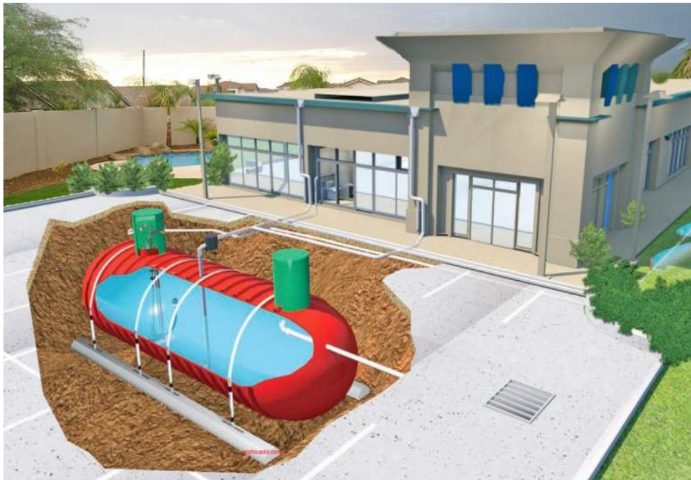
Figure 9.5 – Indicative Rainwater Harvesting Layout
