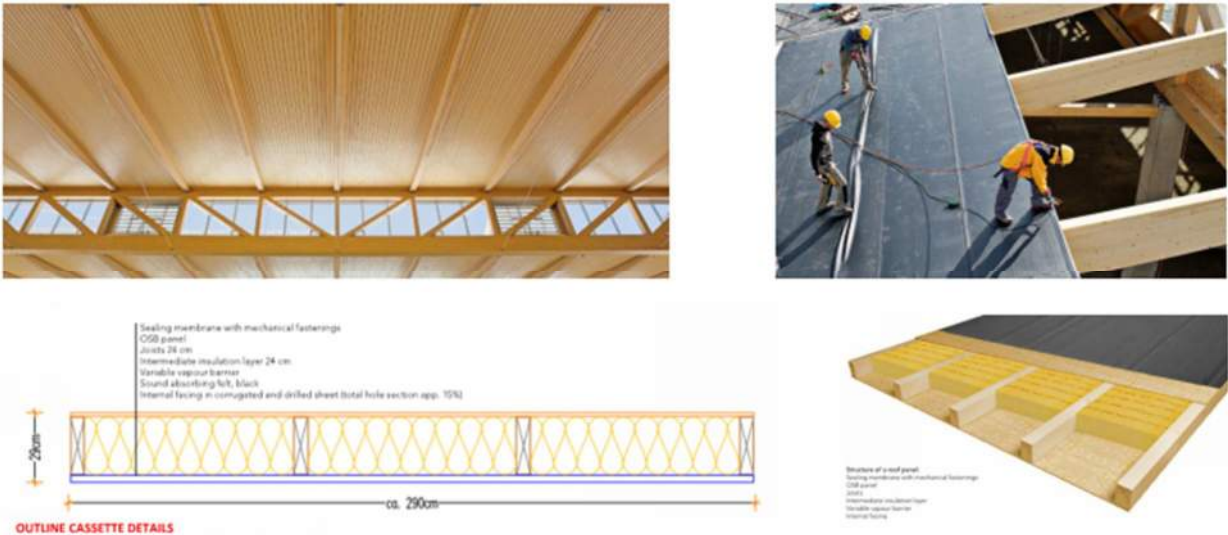
Figure 8.1: Timber Cassette System – Typical Details
