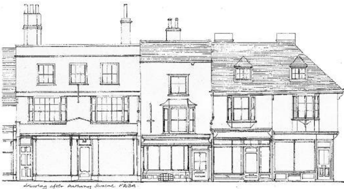
Figure 7 These traditional shop fronts inserted into the ground floors of earlier buildings are variations on the same theme and form a coherent group.
