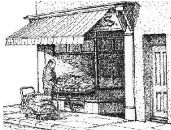
Figure 1 There are two basic types of shop front - those which front the street and have an open window so that customers can select goods directly from them, and those in which the front is permanently glazed, and goods can only be handled within the premises. The former, shown here, is still found but is no longer common. It derives from the open market stall and often tends to colonise the pavement which can add to street vitality.
