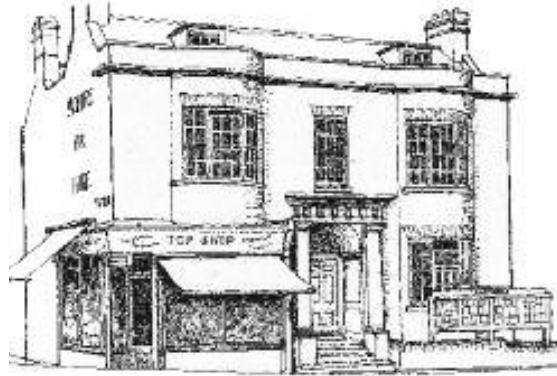
Figure 4 Front inserted into a pre-existing building. The house is of late 18th early 19th century date while the shop front is probably Edwardian. This is a very common arrangement and many examples still survive.
