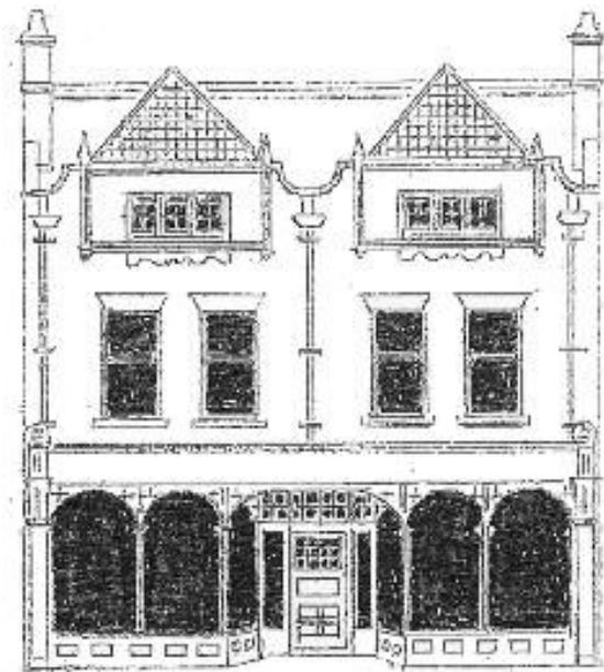
Figure 5 Shop fronts as an integrated part of the original building design. This example shows an Edwardian mansion block with a shop throughout the ground floor. The shop front openings were often clear spanned, which allowed for easy changes at a later date. Iron columns often supported the upper floors.
